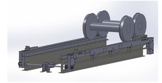
**EMS Solutions** was asked to provide a wheel haulage system to collect rail car wheel sets strewn along a runway and haul them, one wheel set at a time, to a collection point for crane or forklift removal.
