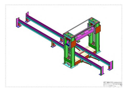
**EMS Solutions** was asked to provide a new high capacity Bogie Press for the disassembly of high load freight Bogies. These bogies are help in place by heavy gauge expansion springs.
